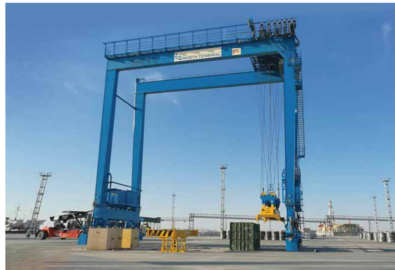
出口哈萨克斯坦轮胎式集装箱门式起重机 Rubber Tire Container Gantry Crane Exported to Kazakhstan
